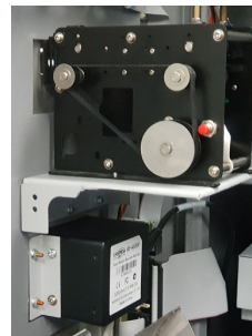
QR Scanner or Motorized barcode ticket/smart card acceptor that provides reliable and speedy ticket/card handling.
